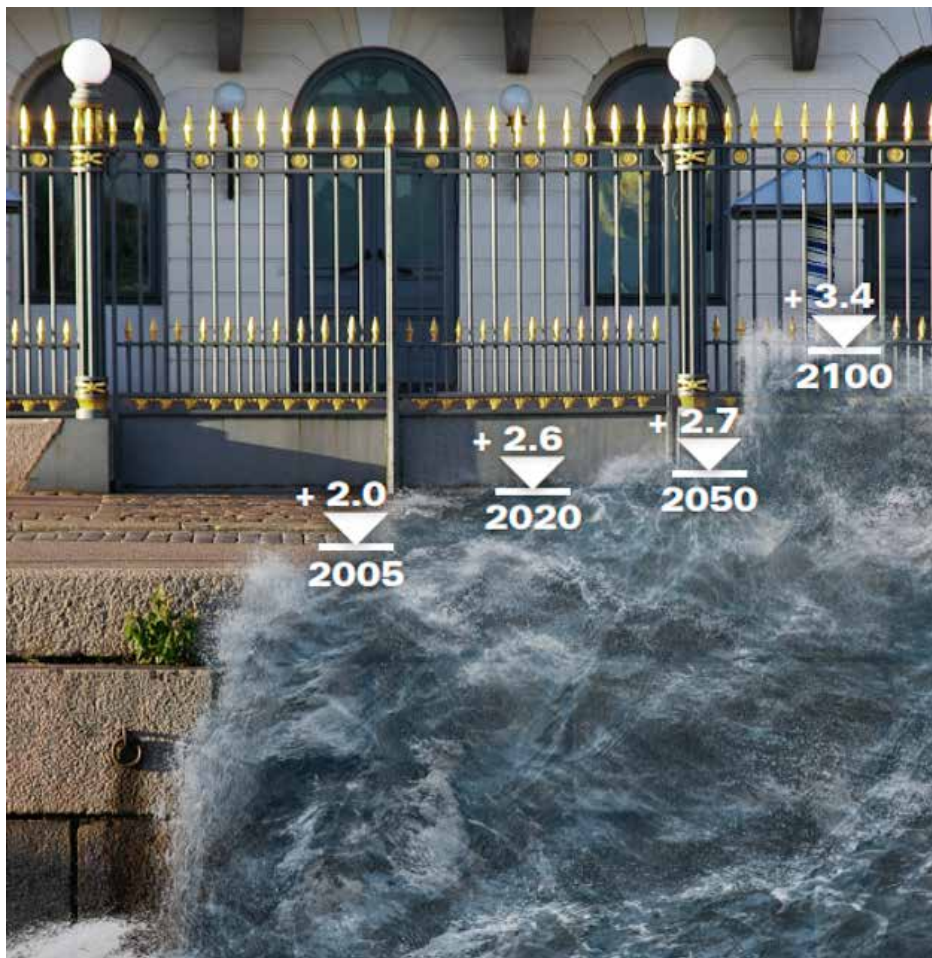
Fig. 28. The flood level measured in 2005 and modelled flood levels in 2020, 2050 and 2100 in front of the Presidential Palace next to Helsinki Market square.
