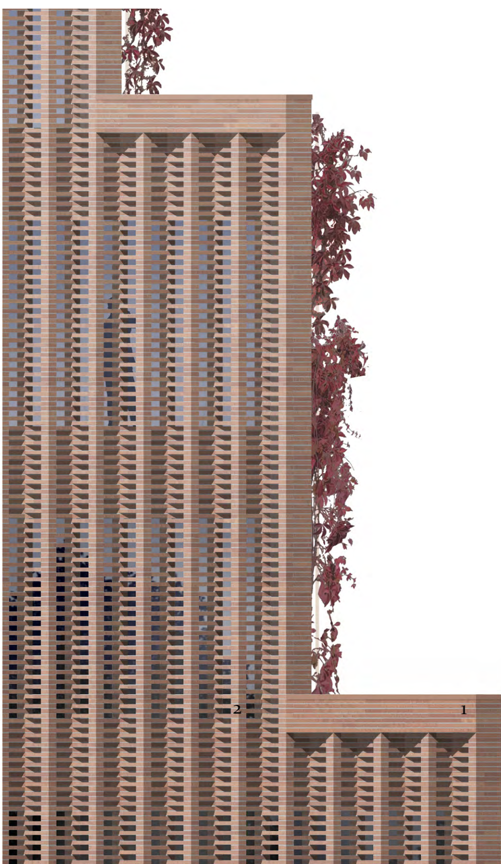
Office facade study, principle of brickwork 1:50
