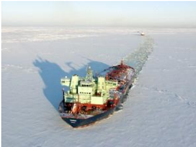
Picture 9: Double acting ice breaking shuttle tanker in action.
