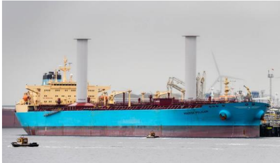
Figure 2: Maersk Pelikan a 110 000 ton oil tanker having two Norsepower installed on the deck.
