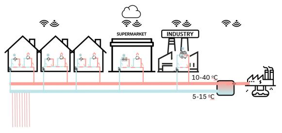
The Local Energy System technology is built on decades of experience from the design, construction and operation of energy systems across multiple countries. It takes the best characteristics of heat pumps and cooling machines and combines them with the best features of energy distribution networks in a new, innovative way.
