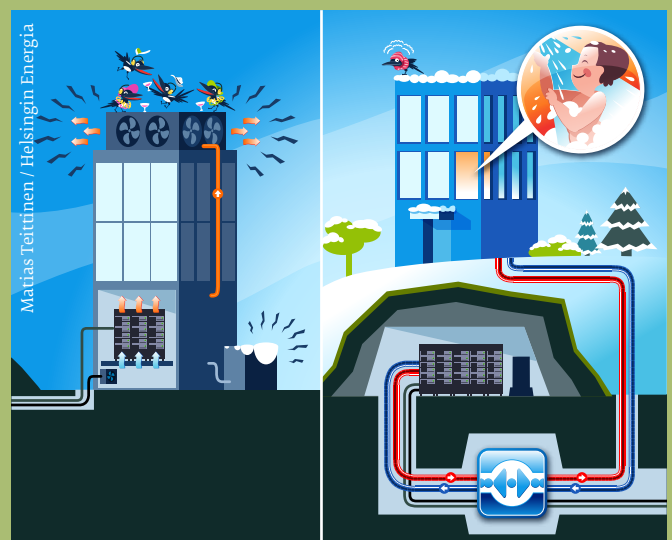
A conventional data centre (left), cooled by a building-specific system, and the new data centre (right), which recovers the heat and is cooled by eco-efficient district cooling.
