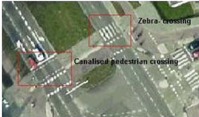
Figure 12: Zebra crossings and a canalised crossing at a same junction in Eindhoven.
