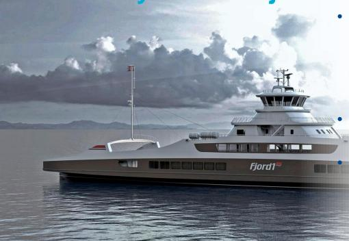
The automatic crossing system ensures safe and energy-efficient transit by automatically controlling the vessel's acceleration, deceleration, speed and track
