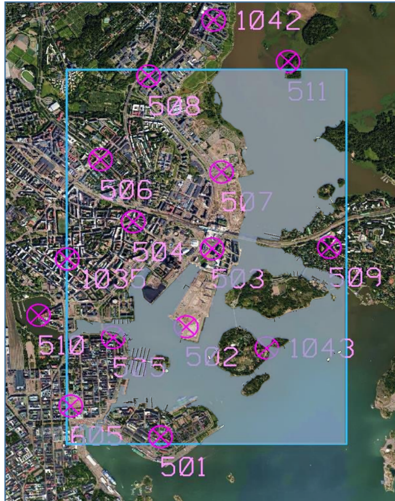
Figure 6. 15 ground control points and waterbodies in Kalasatama
