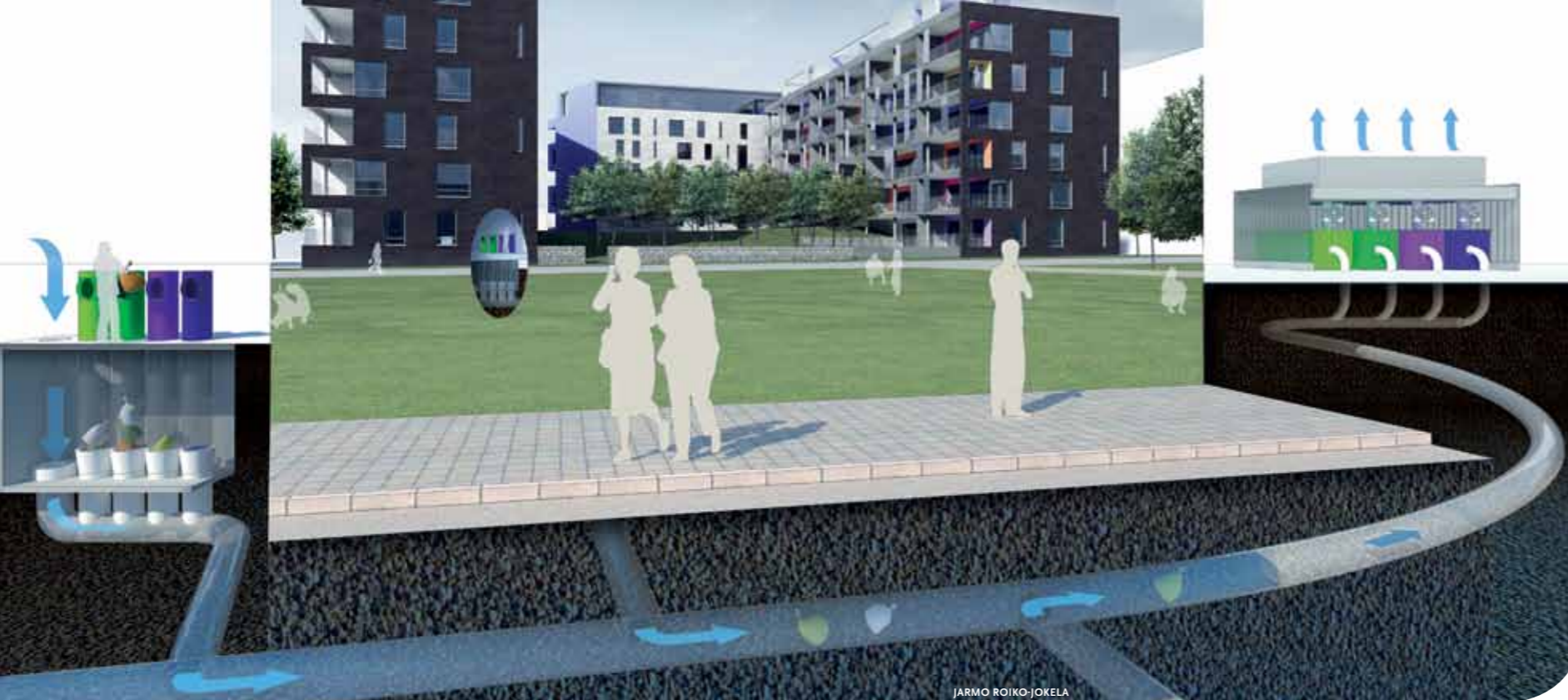
► AN UNDERGROUND PIPE NETWORK, RÖÖRI , will transport domestic waste in the new district of Jätkäsaari into a collecting station. There will be less garbage truck traffic, and the urban environment will remain hygienic and safe.
